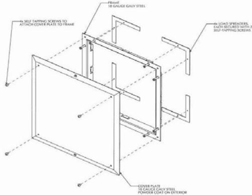
The FSC Inspection Hatch does not require any framing in plasterboard, although existing framing can be used where available.
